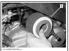
**REMOVE AIR FILTER FROM HOUSING** 1. Air filter
